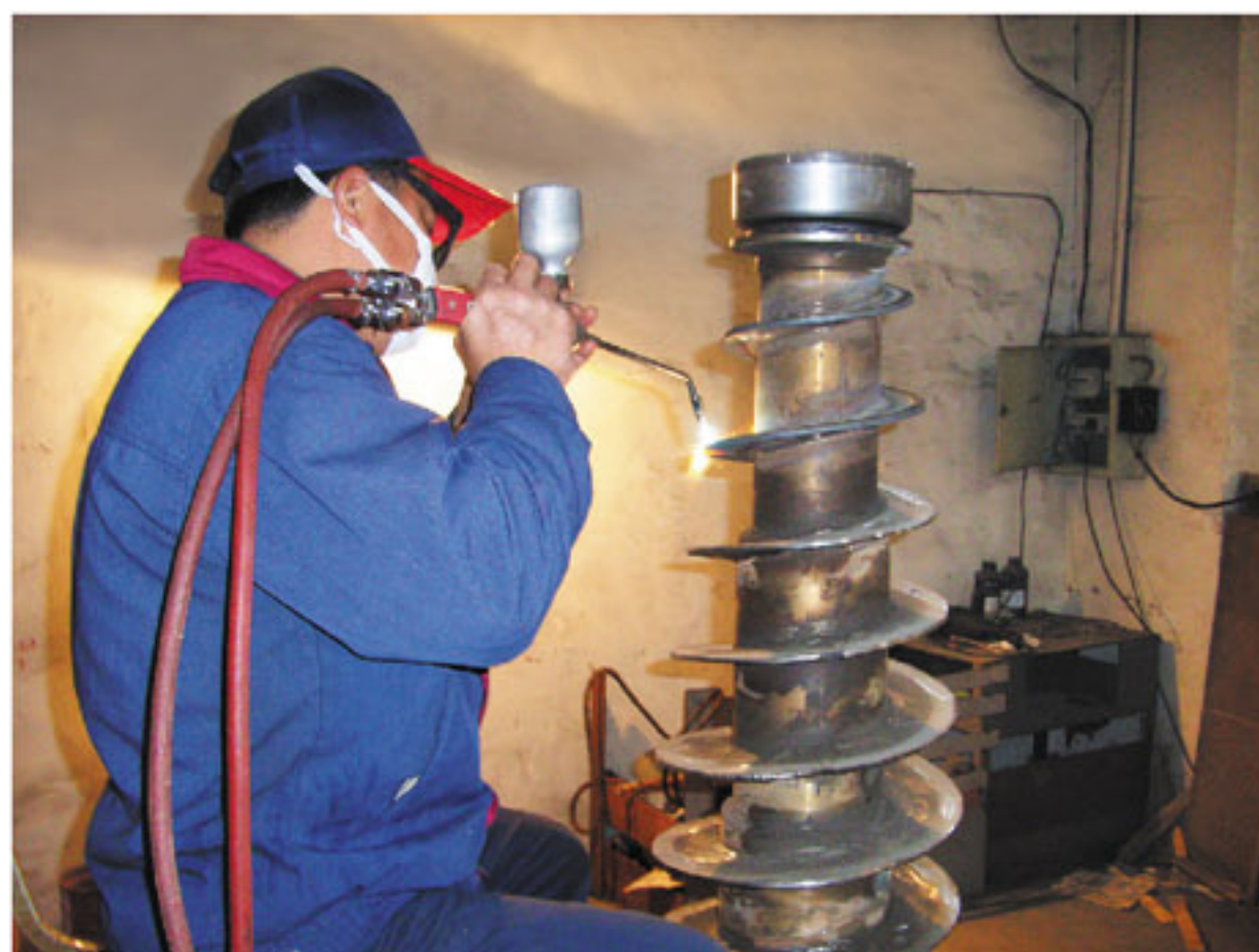
▣ 喷焊硬质合金耐磨层 surfacing welding hard alloy wearing layer
